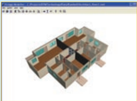
IFC data model from Munkerud project (Norway)
